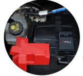
Connect the FINDER via the black plug function to the wiring harness
