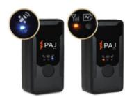
The LEDs flash alternately for 12 seconds
